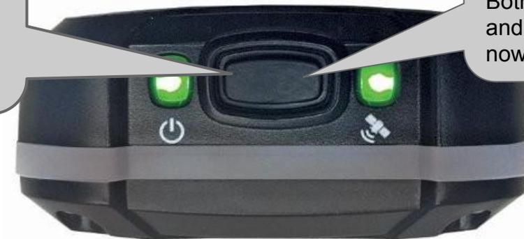
**STEP 2) POWER DEVICE BACK ON.** Briefly press & release the power button. Both lights will flash rapidly and stop. The device is now ON.
